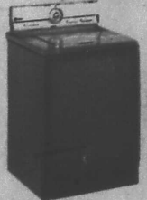
Heavy-gauge zinc-coated steel cabinet. Zinc phosphate paint base, acrylic prime coat and enamel provide rust protection and lasting beauty.
