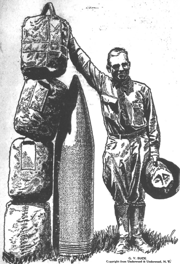
A 14 inch projectile, weighing 1070 pounds, and a charge of 325 pounds of smokeless powder.
